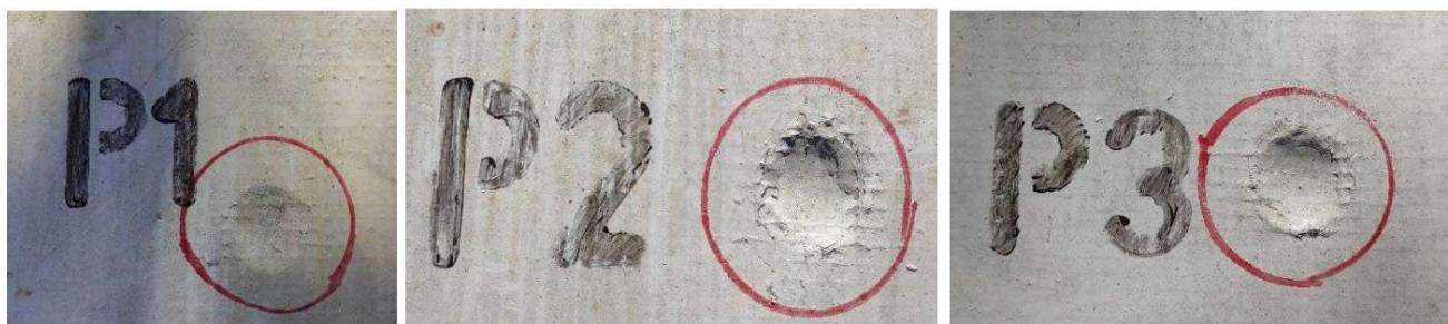
Figure N° 8: Graphical representation of the Steel Ball Impact Resistance Test Method and photography of its imprints
