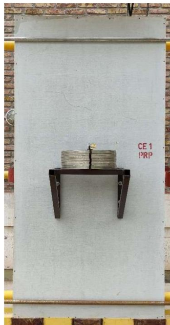
Figure N° 10: Photos of the eccentric load tests
